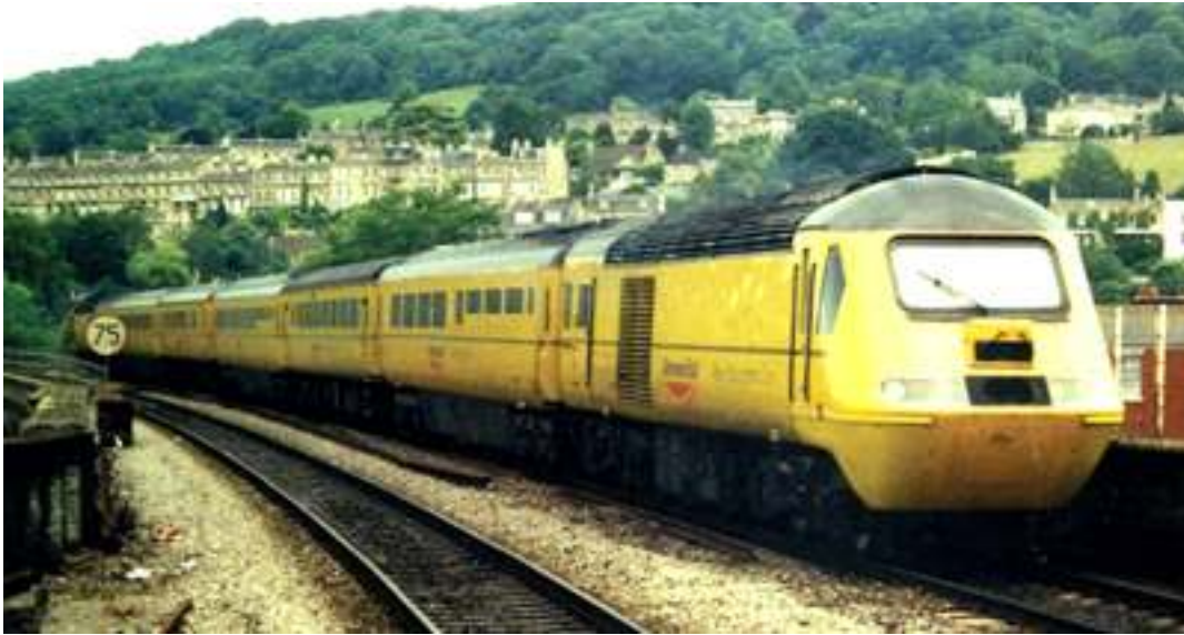
Network Rail's New Measurement Train is crammed with equipment for track geometry data.
